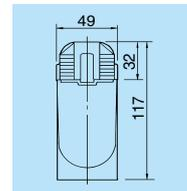
For 300A connections: up to 150mm or 100mm $\times 2$ .
